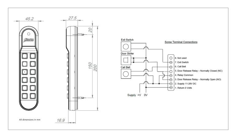
All Storm AXS StrikeMaster Mullion Keypads feature peripheral halo illumination to cast a soft light onto the surrounding surface. This halo illumination feature can be permanently disabled during the installation process if required. The keypads can be specified with either chromed cast metal keytops or white laser marked polymer keytops with integral LED illumination.
