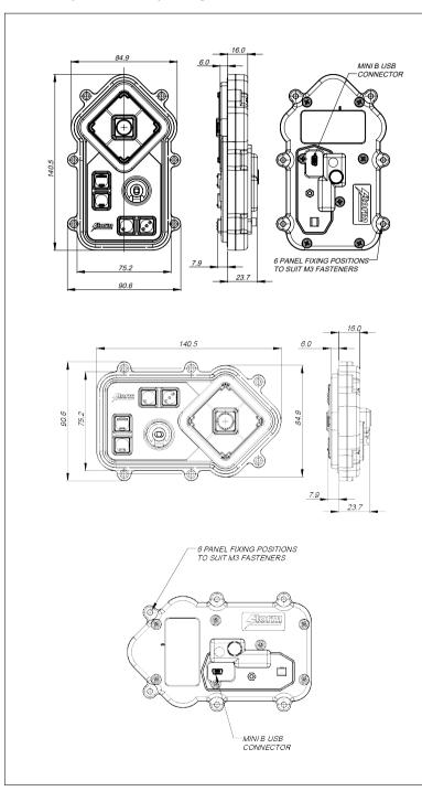
The AudioNav EF is designed for underpanel installation. Both vertical and horizontal versions are available.
