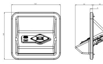
Installation of the AudioNav must be at a height suitable for wheelchair and nonwheelchair users. Ensuring that the AudioNav can be seen and used comfortably by both seated and standing users can be challenging, but the innovative housing of the Angled AudioNav addresses this by presenting the device at an optimal angle.
