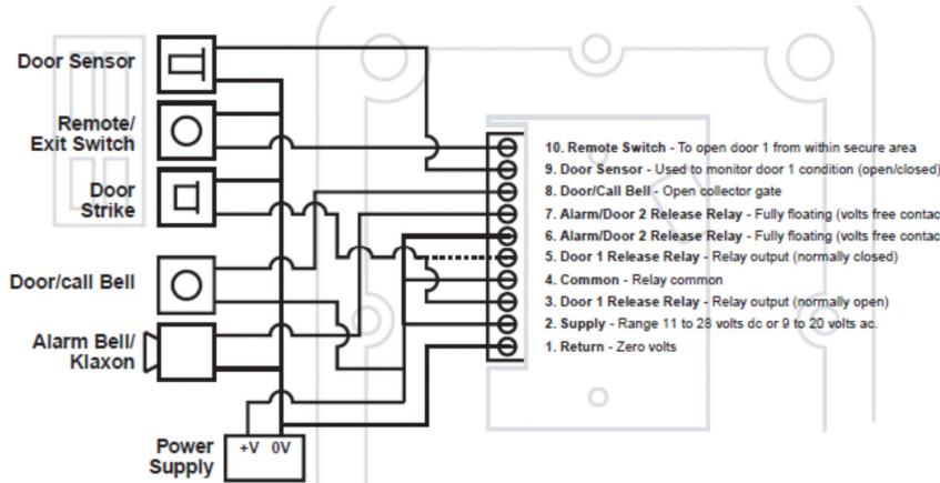
**Note:** When making connection to the door strike, select 'relay normally open' or 'relay normally closed' to suit the intended application and locking mechanism.
