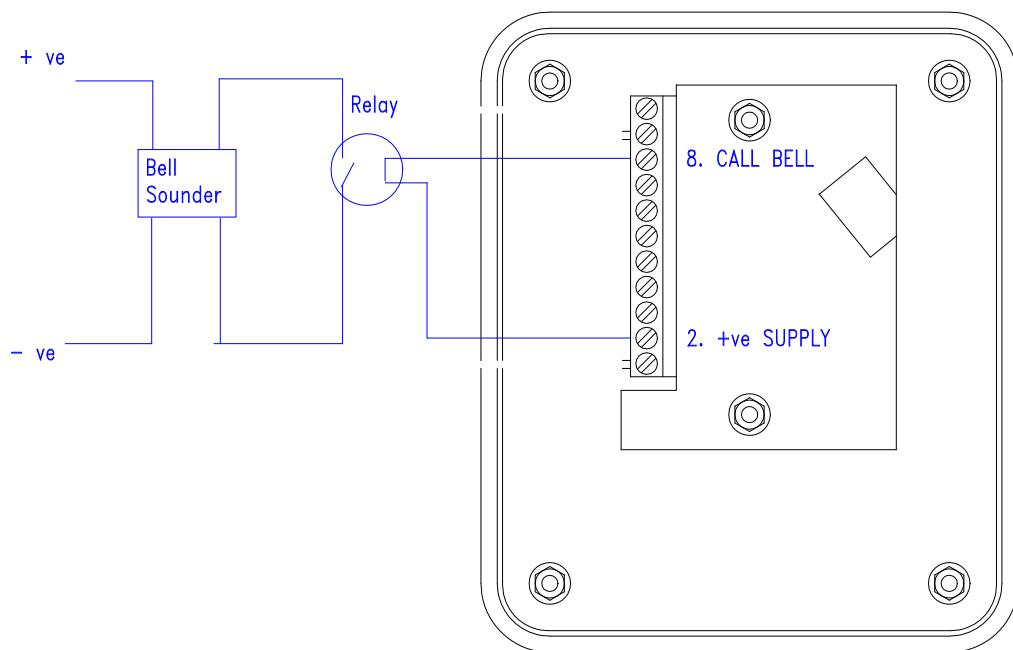
Use a latching relay rated to operate at 60mA, up to 12V dc.
