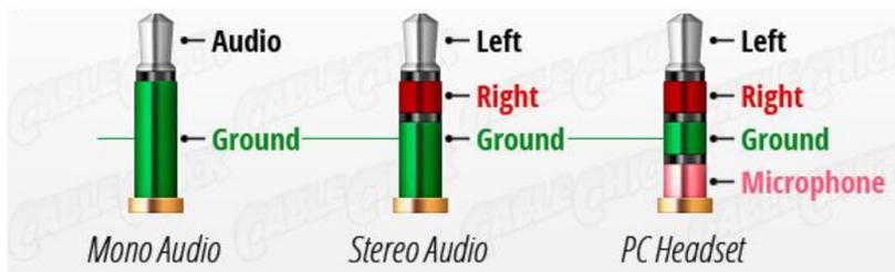
Notes: Application software should always ensure the same audio is present on both Left and Right Channels for correct mono operation. Headsets with microphones can be used. (microphone input is supported on this product)
